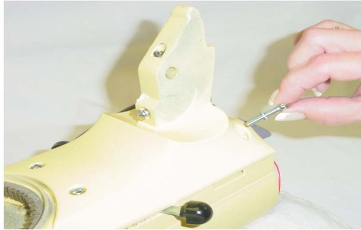
**Fig. 63** Secure the four fillister head screws.
