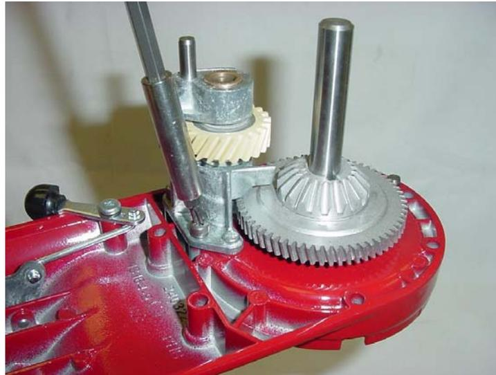
**Fig. 52** Worm gear bracket bearing and pin assembly.
