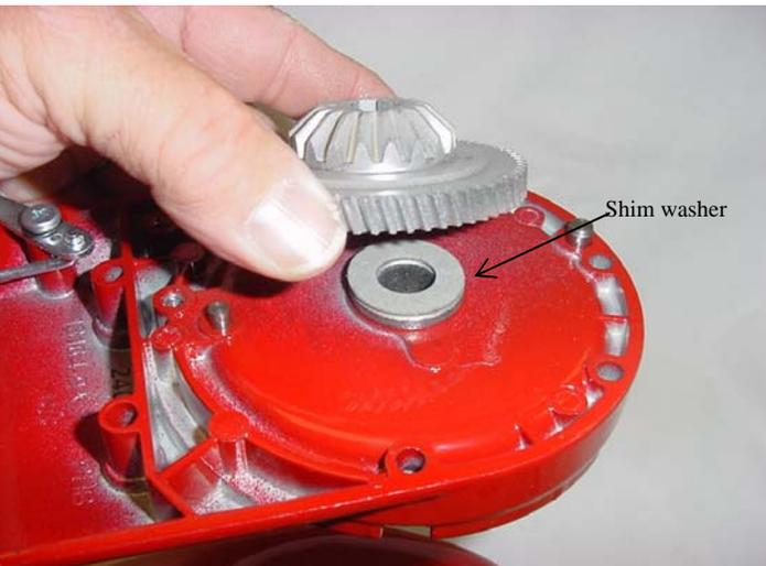
**Fig. 55** Bevel center gear being lifted for inspection.
