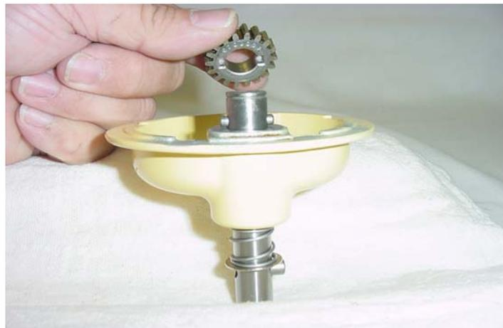
**Fig. 65** Lift the pinion off and take out the pin and remove the washer; then pull out the shaft.
