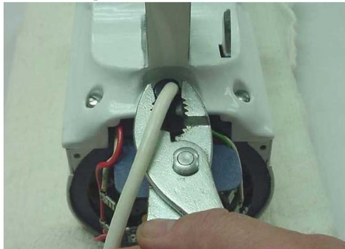
**Fig. 9** Removal of Heyco strain relief using pliers.
