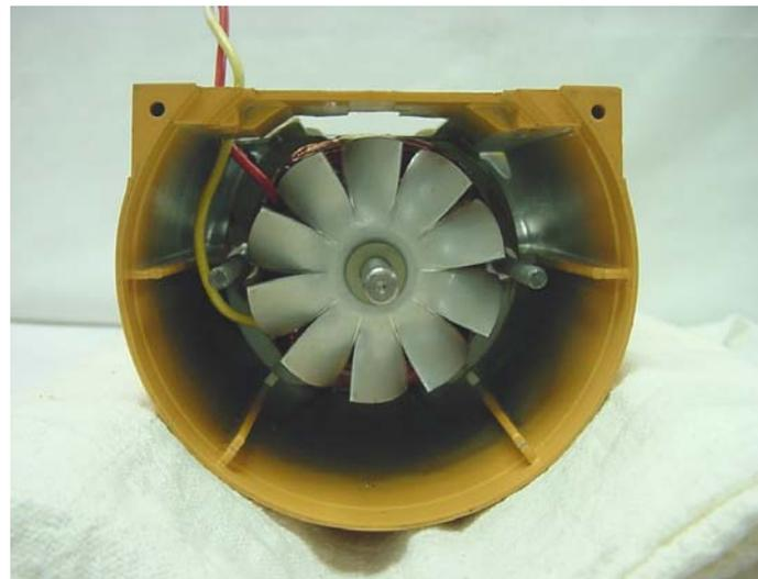
**Fig. 39** Locating the armature into the gearcase-motor housing.
