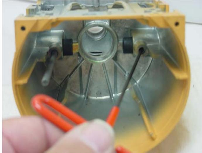
**Fig. 33** Removing the brush holder set screws with a allen wrench.
